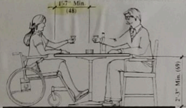
Fig. 23 Accessible tables should provide kneespace at least 2' 2" high by 2' 6" wide with 1' 7" of footroom. To increase the kneespace height, a raised portable leaf can be provided. (See Fig. 24.) Numbers in parentheses are dimensions in centimeters.
